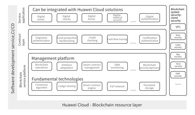
Figure 5-1 BCS Logical Architecture Framework
