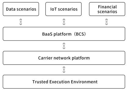
To-be blockchain architecture:end -to-end ;three-in-one;cloud platform+network+TEE
