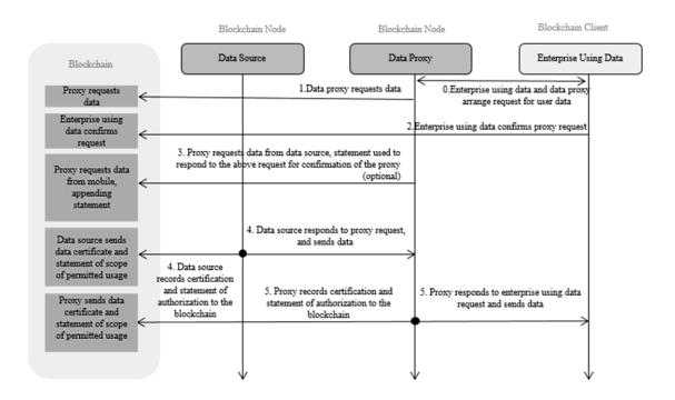
Figure 4-1 Data Exchange Authentication based on Blockchain
